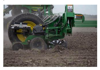
Parallel linkages wear over time, which can lead to excessive movement of the row unit. Bushing wear will tend to make a row unit plant slightly shallower with more tendency for erratic seed distribution. With your planter raised in the air stand behind each row unit and push up and side to side. If you find that the row unit moves excessively, it is time to replace the parallel linkage bushings.
