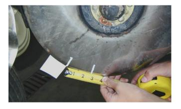
Depth-gauge wheels should be checked to make sure that they turn freely, move up and down easily, and run tightly against the opening discs. This is important to ensure that soil doesn't flow between the wheels and the opening discs and into the seed trench, which can result in irregular seed placement and planting depth variability. Yearly inspections will tell you if the gauge wheel arm bushings are worn and if the wheels need to be shimmed in against the double disc openers.
